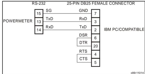
**Figure 2-16** RS-232 Simple 3-Wire Computer Connection, 25-pin
