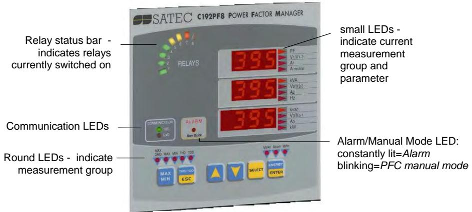
The front panel display is updated approximately twice per second; you can adjust the display update rate via the *Display Setup Menu* (see Section 4.8).
