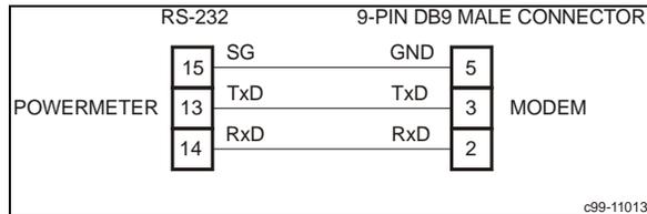
**Figure 2-15** RS-232 Connection for 9-pin Modem Connector
