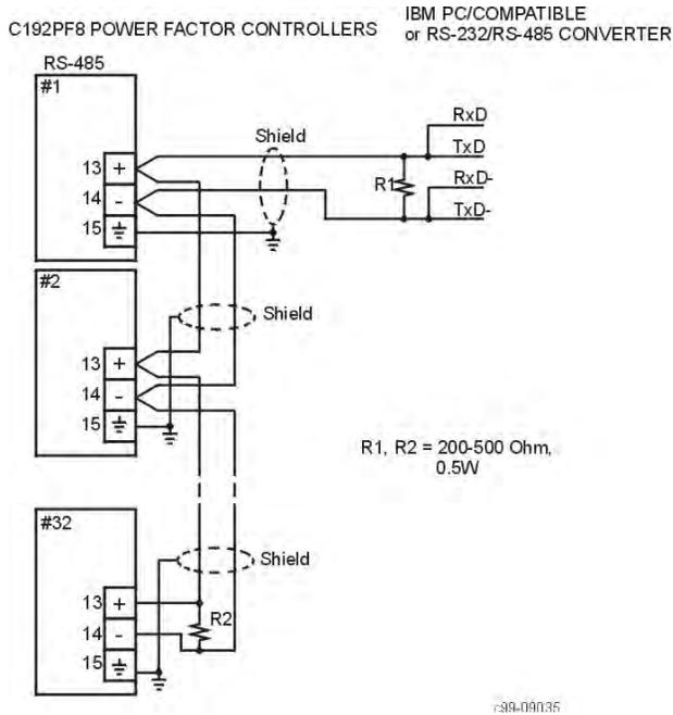
**Figure 2-18** RS-485 Multi-drop Computer Connection
