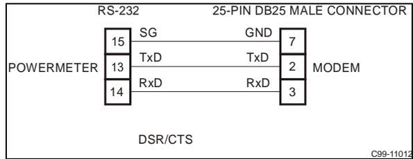
**Figure 2-14** RS-232 Connection for 25-pin Modem Connector
