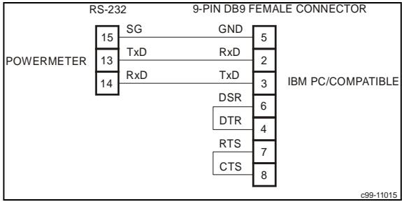
**Figure 2-17** RS-232 Simple 3-Wire Computer Connection, 9-pin
